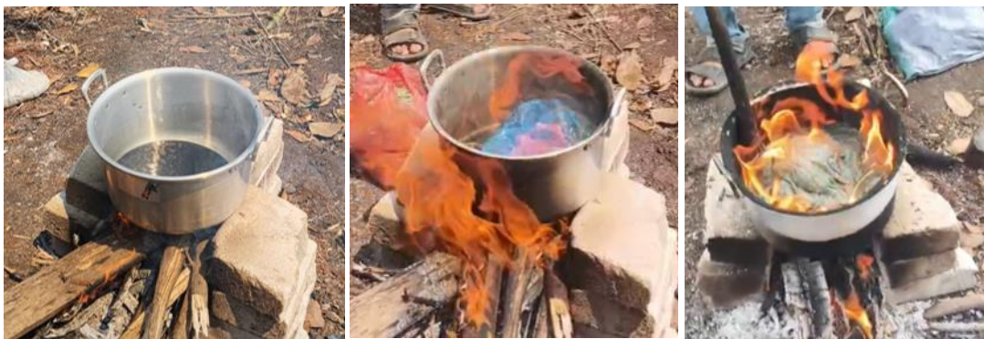
Gambar 1. Proses Memasak Adonan Paving Block
