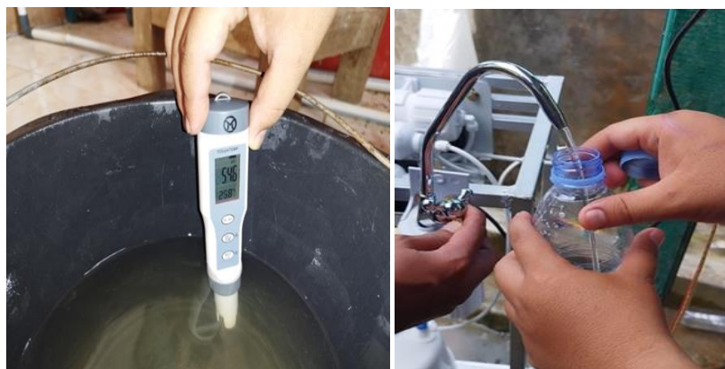
Figure 4. Water Trans Malakoni RO water sample before the treatment process and water after the RO process
